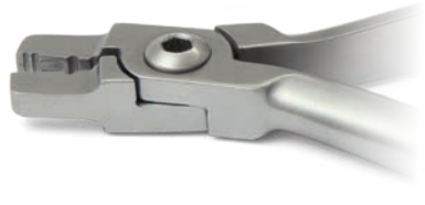
ZLH508 Pinza per archi linguali - Lingual arch plier ● Per piegature doppie o triple - To form double or triple back bends in wires ● Max 0.030" (0,76 mm); 0.036" (0,91 mm)
